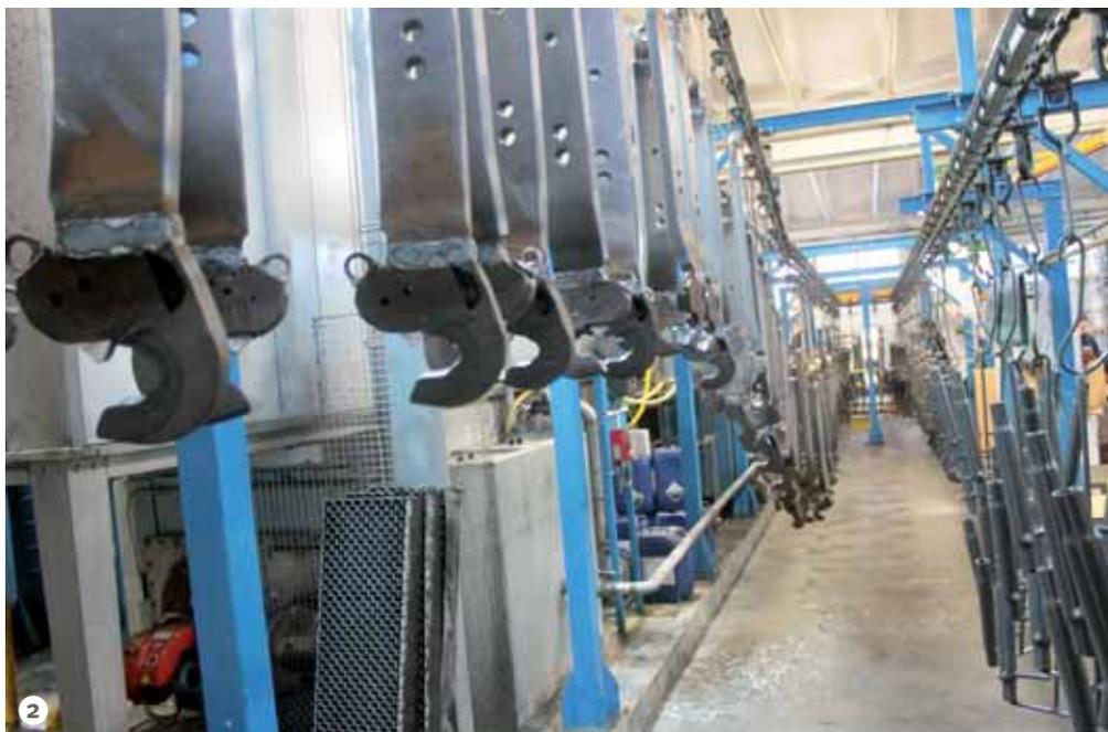
**Figure 2: The monorail conveyor leads the hydraulic cylinders along the pre-treatment and coating line.**
