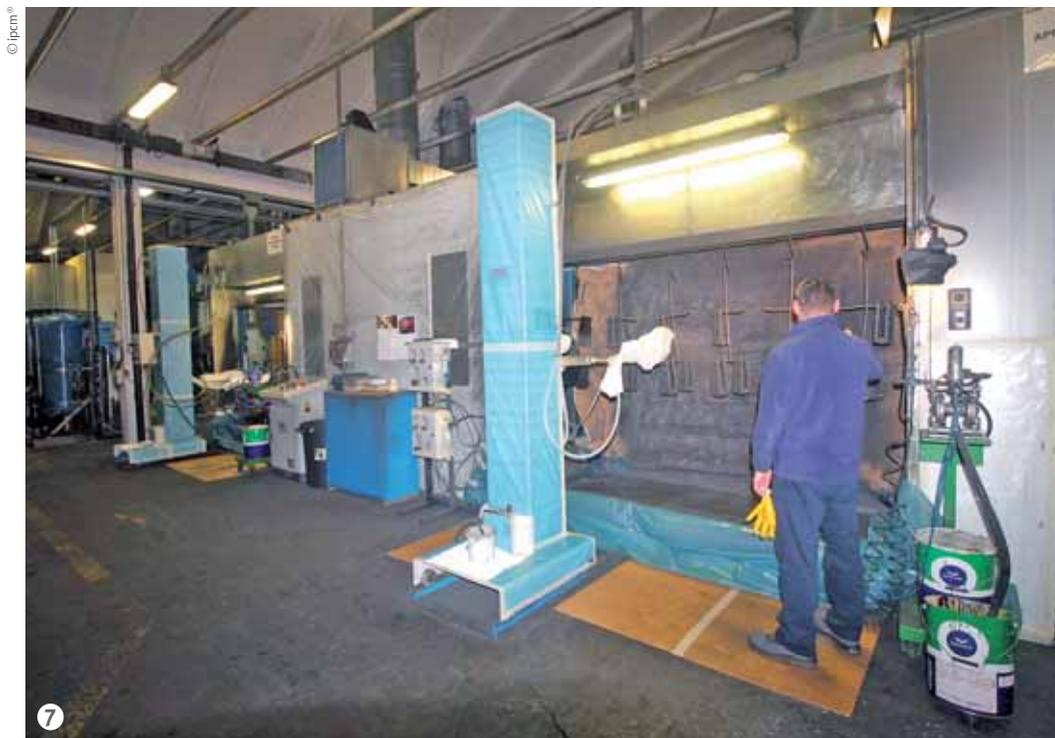
Figure 7: The two booths for the dry application of primers and topcoats.
